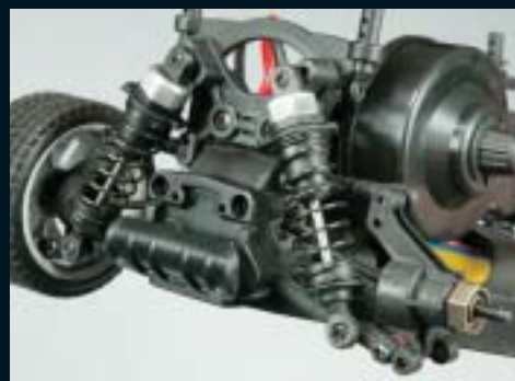
Big-bore oil-filled shocks soak up the bumps. Check out the beefy hub carrier.
