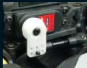
The 1/10 servo offers more options and will allow future upgrades. A servo-saver is built into the servo horn and has plenty of adjustment options.
