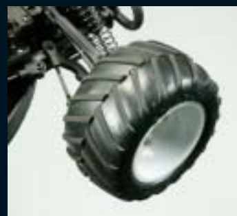
The truck version has dish-type wheels with chevron-tread tires.
