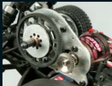
The fully adjustable slipper-clutch system allows you to adjust the power transfer from the motor to the wheels.
