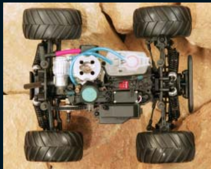
The MG16 comes neatly laid out and easy to work on. Note the tube that connects to the muffler. This carries away exhaust fumes and fuel, helping keep the MG16 free of dirt and debris.
