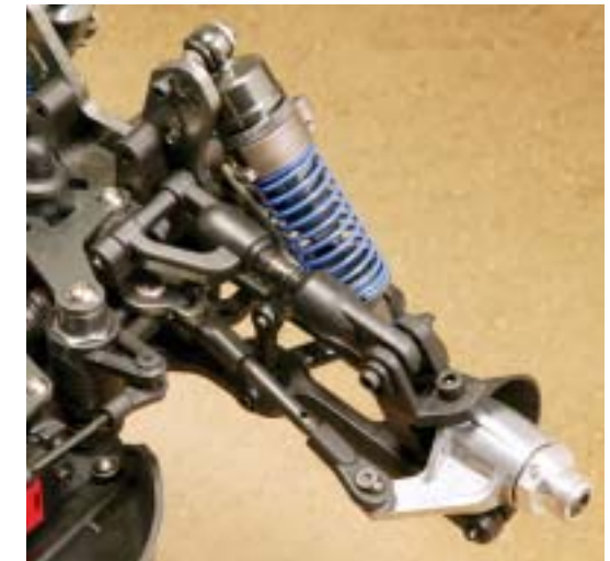
CEN went with a C-hub front suspension setup with 22° caster blocks and large oil-filled shocks with 3.5mm shock shafts, all of which lets this buggy handle bumps with ease.
