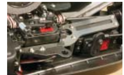
To keep the CG low, the steering servo lies down and bolts up under the aluminum servo tray. Fitted to the radio tray is a transponder mount for regular transponders. Another feature to note is the narrow mudguards that give the buggy its narrow stance.
