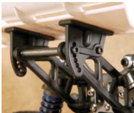
Normally you only see two to three holes to adjust a rear wing, but the Matrix has six different positions. The supports are farther apart for better stability and have aluminum braces.
