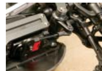
The main bellcrank houses a servo saver with an aluminum drag link to connect to the other crank. Several holes on the drag link allow you to move the steering links and alter its action.
