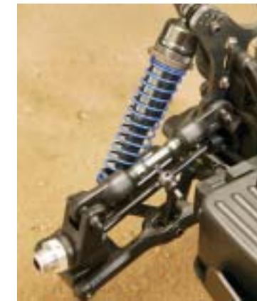
CEN went with a C-hub front suspension setup with 22° caster blocks and large oil-filled shocks with 3.5mm shock shafts, all of which lets this buggy handle bumps with ease.
