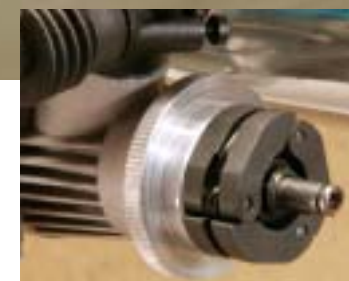
A 3-shoe composite clutch and aluminum flywheel transfer power to the drivetrain.
