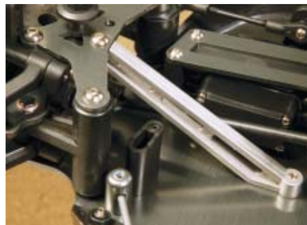
Normally you only see two to three holes to adjust a rear wing, but the Matrix has six different positions. The supports are farther apart for better stability and have aluminum braces.
