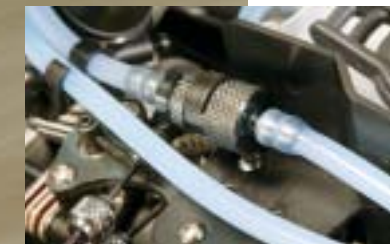
Here is a nice feature on the Matrix: the included fuel filter that attaches to the splash guard that keeps spilt fuel from contaminating the brakes.
