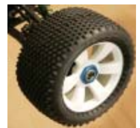
Lightweight six-spoke wheels are shod with effective block-tread rubber tires. 23mm hex drives are more durable than standard 17mm hexes, although it may be harder to find suitable replacement wheels.
