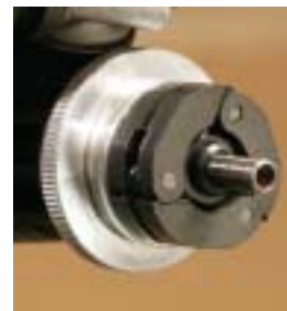
A three-shoe composite clutch grips the 13-tooth steel clutchbell. Firmer clutch springs would improve performance by delaying engagement until the engine built more revs.
