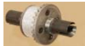
All three diffs have hardened-steel bevel gears, aluminum cases, and six internal gears. The internal pinion gears are caged to improve the diff's limited-slip capabilities.
