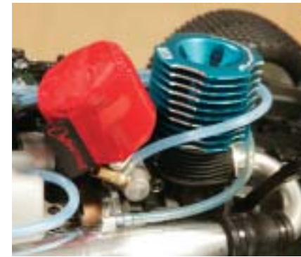
CEN's powerful new TR .28 engine ran flawlessly for our test. We installed an Outerwears filter skin to extend the time between filter cleanings.
