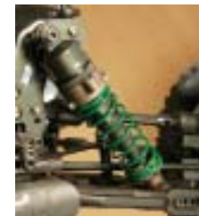
Dual-bellcrank steering features an integrated, spring-loaded, adjustable servo-saver. The 3mm aluminum steering plate offers three Ackerman choices.
