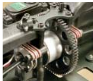
The beefy, aluminum-cased center diff is spun by a CNC-machined 66-tooth steel spur gear. Four vented-steel brake discs provide stopping force.
