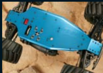
What sets the Magnum apart from its predecessors is a new, one-piece aluminum chassis, which replaces the old MT2's two-piece affair. The new design is far stronger.
