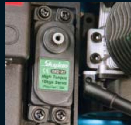
The included Skyion high-torque throttle/brake servo pumps out a whopping 100 grams of torque, and its metal gears guarantee it will be able to do it time after time.
