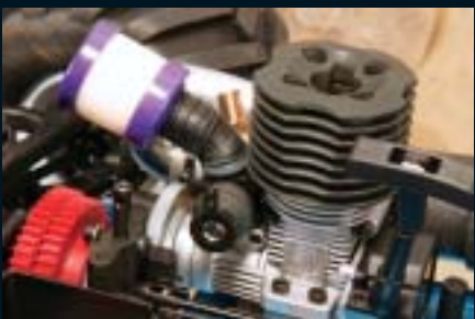
Nestled into the Magnum NX is CEN's powerful .18 mill with pull-start, rotary carb, foam air filter to keep out dirt and large, black heatsink head.
