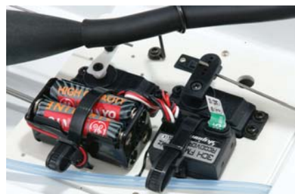
A 2-channel, 27MHz FM radio system with 2 standard servos is already installed but it's somewhat exposed. I did get water inside the hull at times, but it did not seem to affect the gear.
