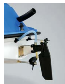
The large, in-line rudder does a great job of steering the Shark. The tube that's visible here is the water pick-up that sends water around the engine for cooling and then exits at the side of the hull.
